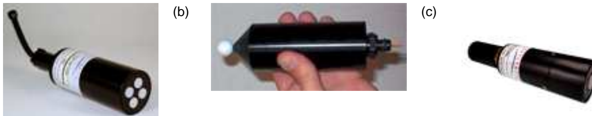
Figure 8 Radiance and irradiance sensors (a) deployable on gliders: (a) the Satlantic Irradiance/Radiance sensor OCR504 (Satlantic 2013c), (b) the Biospherical Instruments PAR sensor, QSP 2000 series, (c) the Satlantic PAR sensor (Satlantic 2013c).
