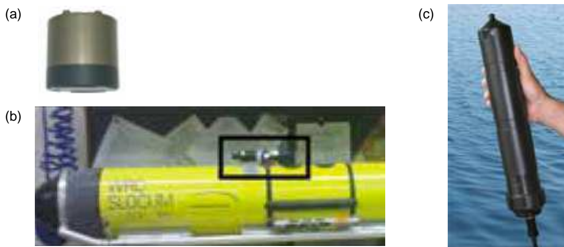
Figure 9 (a) The Imagenex 853 Echosounder (Imagenex 2013), (b) A VEMCO Mobile Transceiver (VMT) mounted on a Slocum glider (Oliver et al. 2013), (c) The VEMCO cabled receiver VR2C (Denise King, personal communication).
