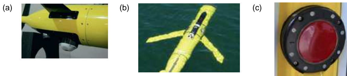
Figure 7 (a) A Nortek AD2CP integrated on a Seaglider (Nortek 2011), (b) A Nortek Aquadopp on a Slocum glider (Rusello 2012), (c) A Teledyne RD Instruments Explorer DVL mounted on a Slocum glider (Jones et al. 2011).
