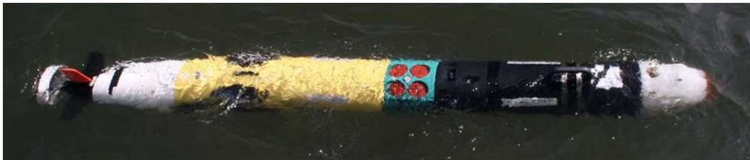
Figure 16 A prototype MarChem sensor (configured for use as an NRL/SubChem Systems ordinance immunosensor) deployed on a REMUS 100 AUV (Hanson and Kusterbeck 2010).
