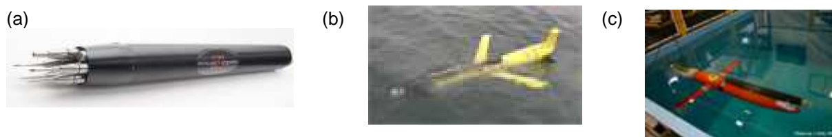
Figure 11: (a) The Rockland SI MicroRider-1000 (Rockland Scientific 2013a), mounted on (b) a Slocum glider (Rockland Scientific 2013a), and (c) a Spray glider (Rockland Scientific 2013b)
