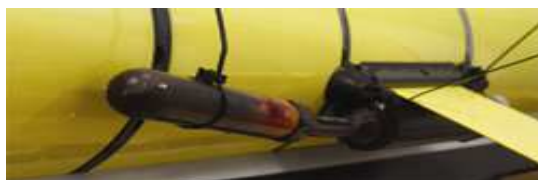
Figure 12: An Acousonde recorded mounted externally on a Slocum glider (courtesy Pierre Cauchy).
