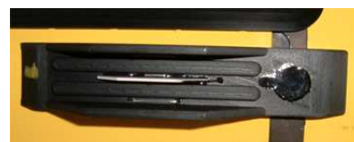
Figure 3: (above right) The fin-cell GCTD mounted onto a Slocum glider (Schmitt and Petitt 2006)
