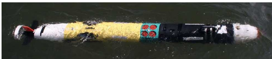
Figure 15: A prototype MarChem sensor (configured for use as an NRL/SubChem Systems ordinance immunosensor) deployed on a REMUS 100 AUV (Hanson and Kusterbeck 2010).
